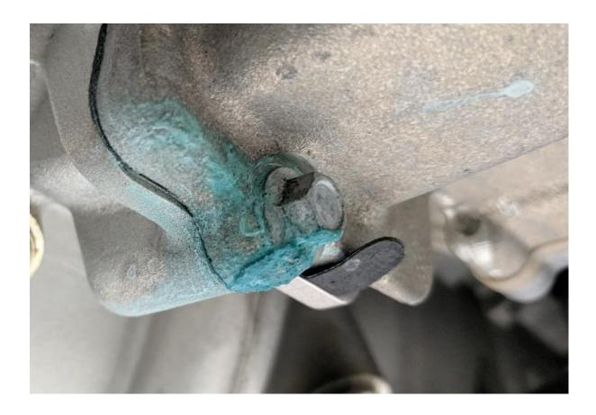
3. The rear of the coolant pump where there is a blanking plug which covers the rear evaporation chamber of the pump.
