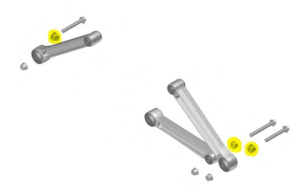
If is confirmed that the spacer is the cause of the noise, remove the retaining bolt and check if the spacer is loose fitting in the engine frame as per the video below.
