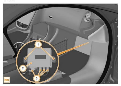
1. Install the two missing fixing bolts (2) and torque to 6 Nm to retain the footrest to the tub.
